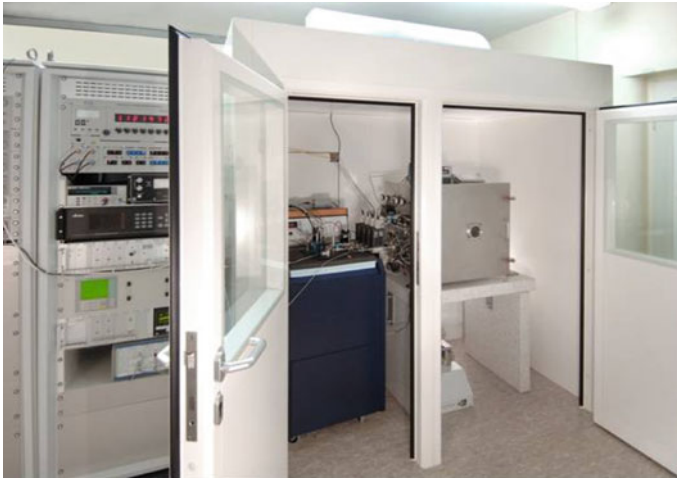
Fig. 3 Constant-temperature chamber with thermostat ( left ) and weighing chamber ( right ) and electronic control unit and data acquisition system outside the chamber
